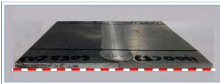
Figure 12: Joint free from distortion
